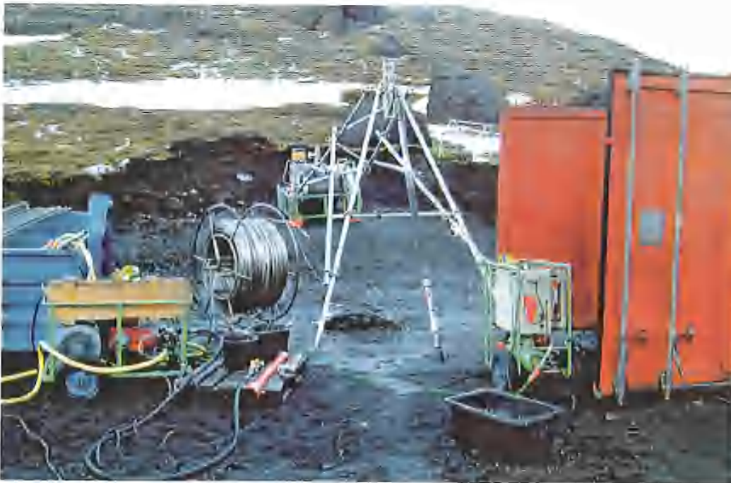
Figure 2.1: Photo showing the MeSy winch system MKW-500, the straddle packer tool PERFRAC II and the injection pumps at the location of well JB-17.
